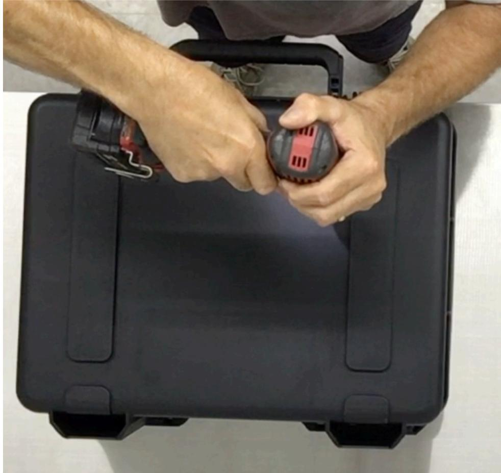
**Step 16** Remove the Slider plate from the case. Use the  $21/64$ " drill bit and electric drill to enlarge the  $1/4$ " pilot hole.
