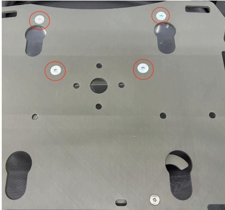
**Step 24** Re-install the plate onto the bike using the M8 flat head screws and lock nuts.
