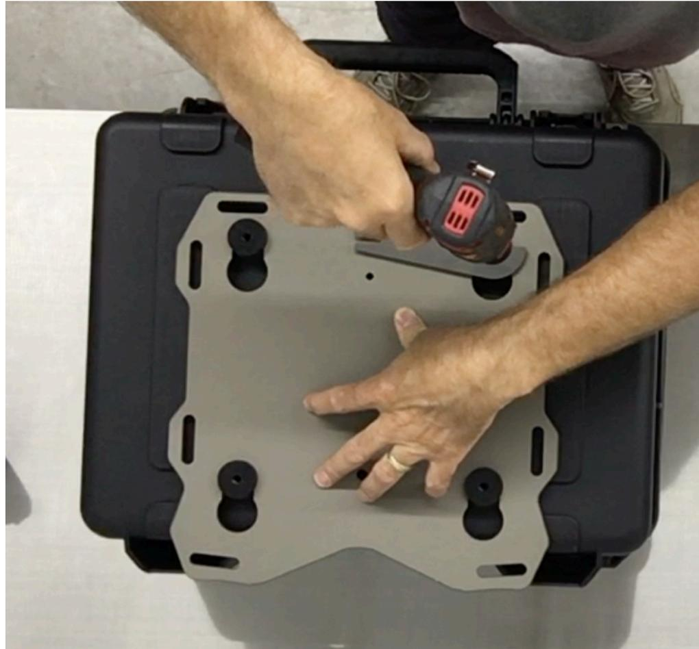
**Step 15** With one hand apply downward force on the Slider plate, use your other hand to drill the case. With a ¼” drill bit and electric drill use the master puck as a drill guide and drill a pilot hole through the box.
