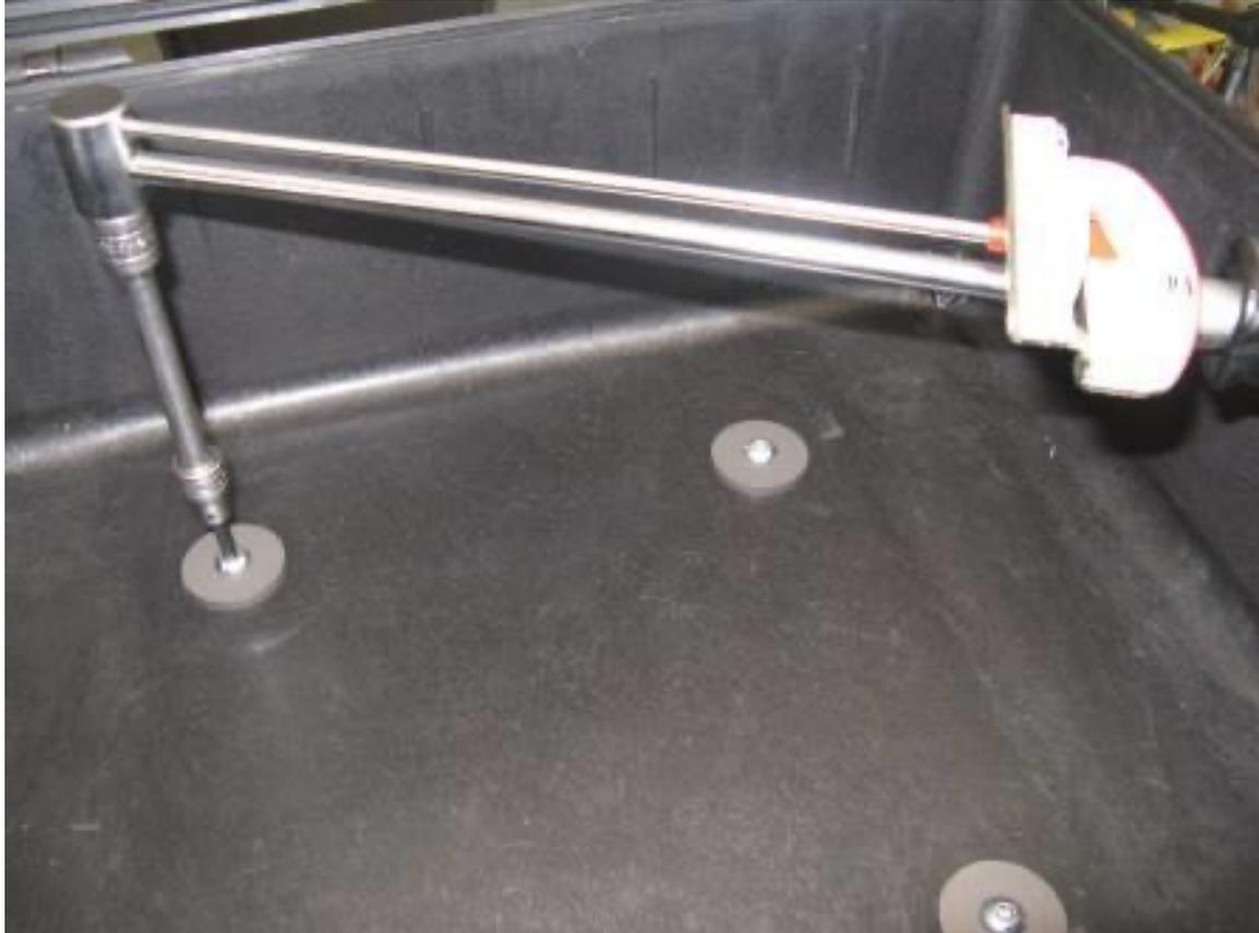
**Step 27** Torque the puck screws to 9 ft.lb. or 12.2 Nm.
