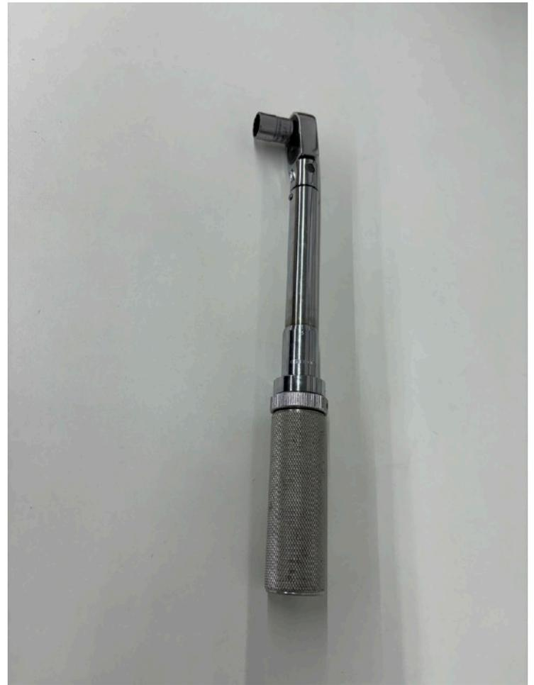
**Step 25** Thread an M8 lock nut onto each of the M8 flat head screws. Use a M6 hex wrench to hold the flat head screws and use a torque wrench to torque the lock nuts to 26 Nm (19ftlb).
