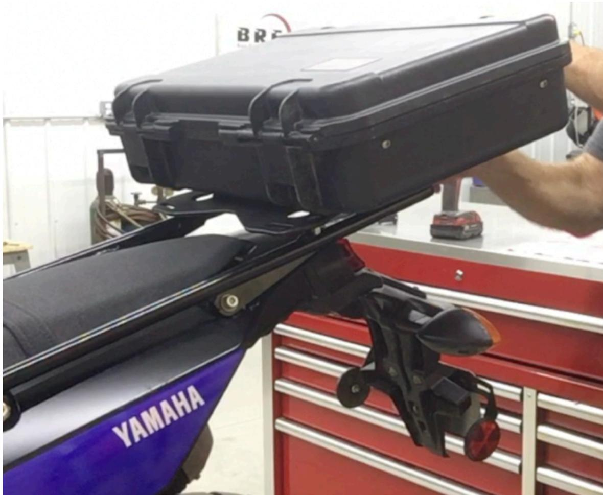
**Step 26** Install the case onto rack and latch it into place with the cam lever.
