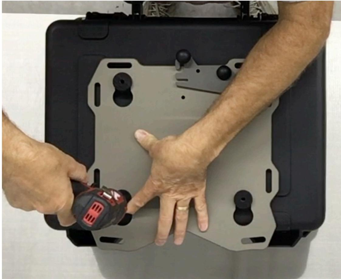
**Step 19** With the ¼” drill bit, use the puck diagonally across from the master puck as a drill guide and drill a second pilot hole in the case.
