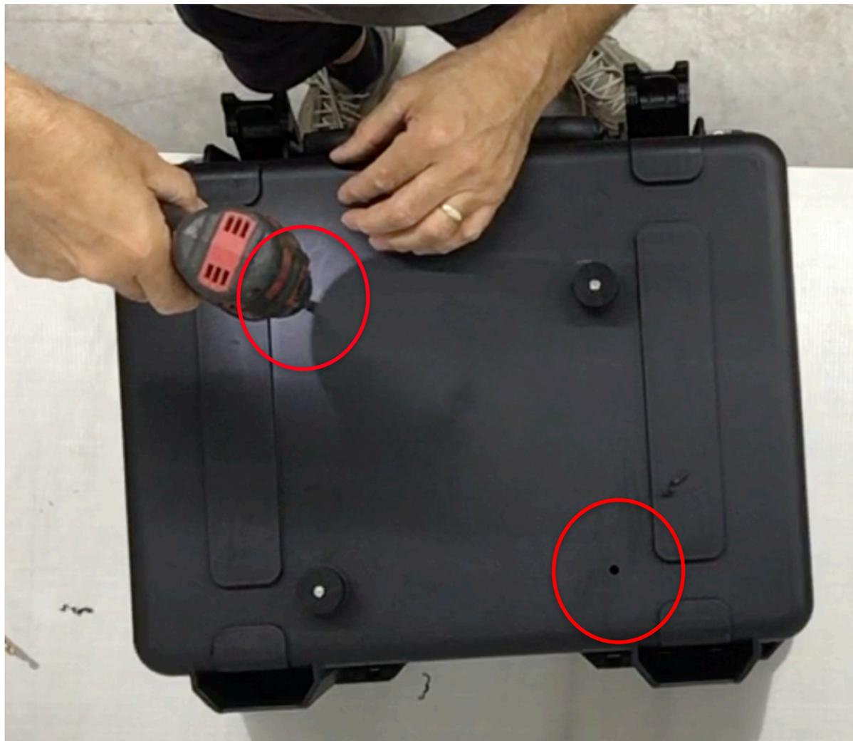
**Step 22** Remove the Slider rack and pucks from the case. Use the  $21/64$ " drill bit and electric drill to enlarge the last  $2\ 1/4$ " pilot holes.
