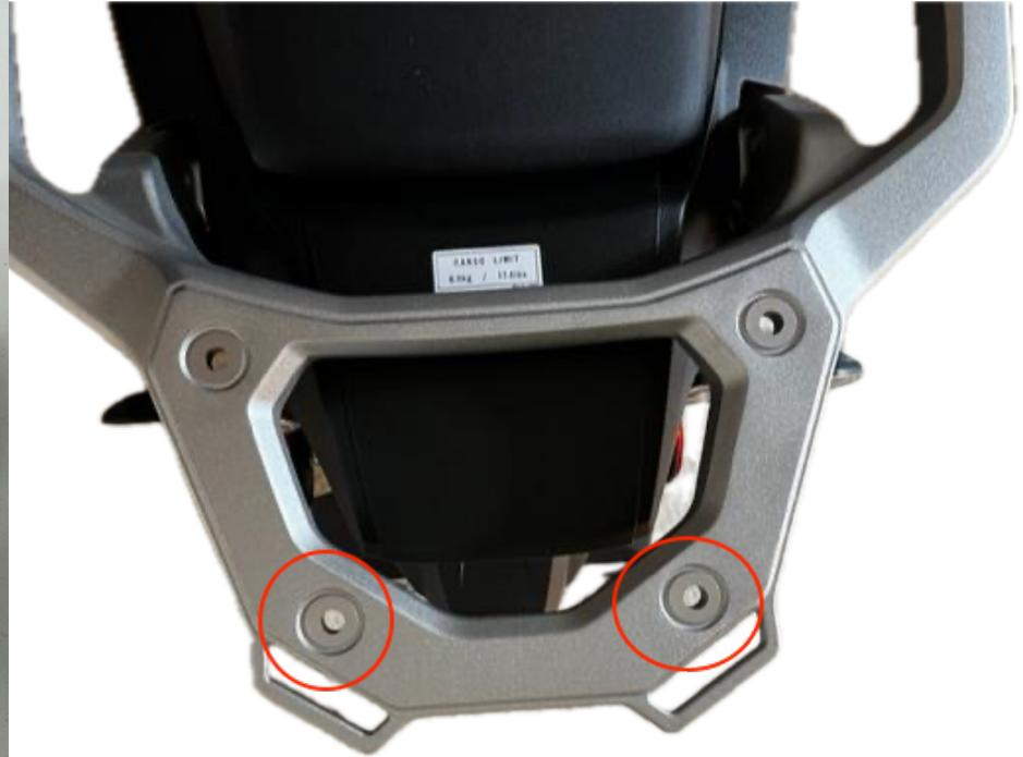
**Step 2** Stack the 41 x 5 mm aluminum spacers on top of 22 x 8 mm aluminum spacers. Place a spacer stack over each of the rear holes as shown. **Note:** Make certain the uncoated side of the large diameter spacer faces upward toward the Slider plate.
