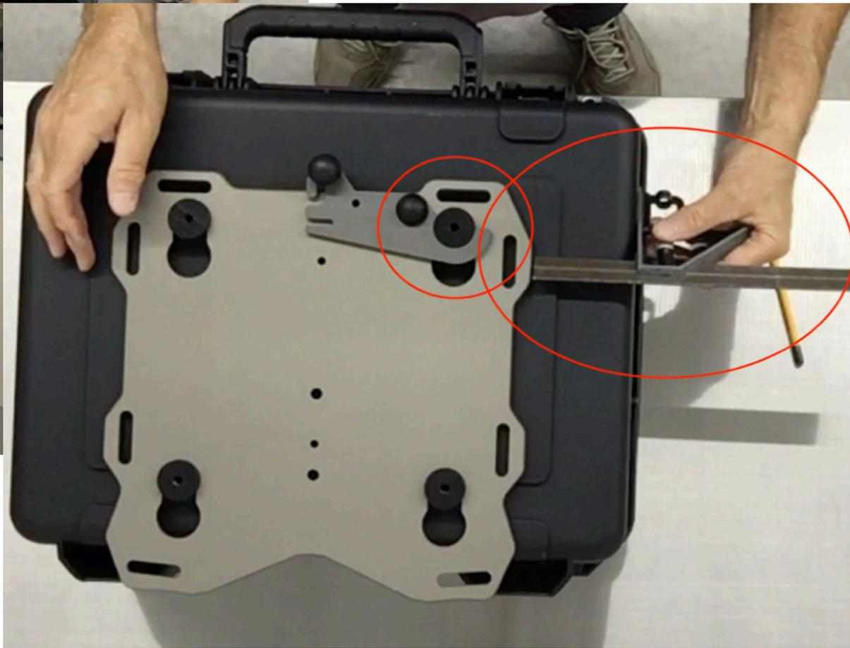
**Step 14** Locate the puck marker on the case and align the master puck with the mark as it was on the bike. Adjust the box side to side and make any final adjustments to the location.
