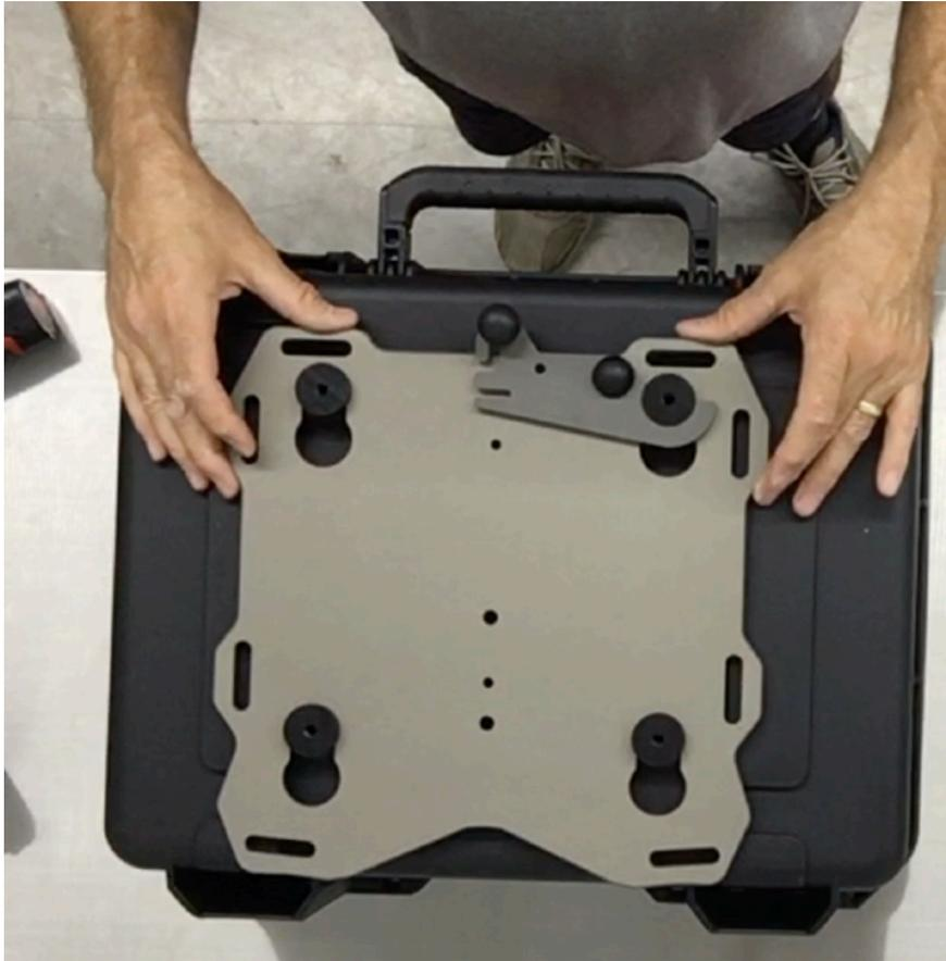
**Step 13** Place the case on a table or other work surface. Remove the 4 flat head screws and nuts holding the Slider plate onto the OEM rack. Place the Slider plate with the pucks installed on the case.
