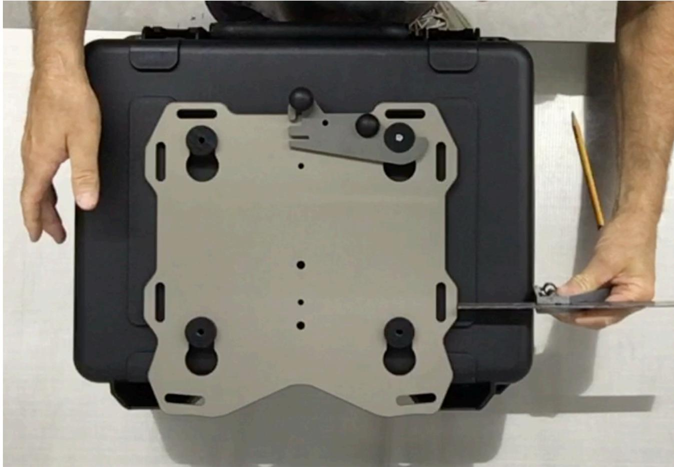
**Step 18** Place the Slider plate with the other 3 pucks onto the master puck and latch it into position. Square up the plate and box to each other (last chance).
