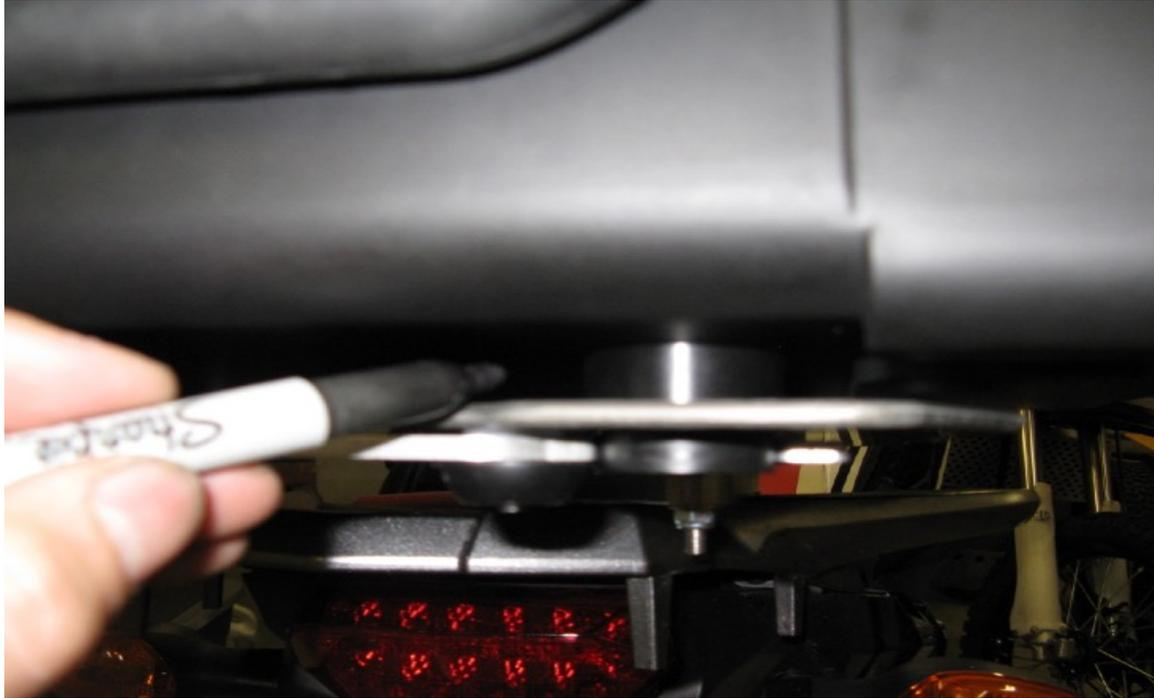
**Step 12** Position the case on top of the pucks. Determine the for/aft location (side to side will be determined later). Position the box as far forward as possible without interfering with passenger comfort. Also consider if you will be placing any gear on the seat or if you want to be able to remove the seat with the box in place. Use a marker to mark the master puck location on the box.
