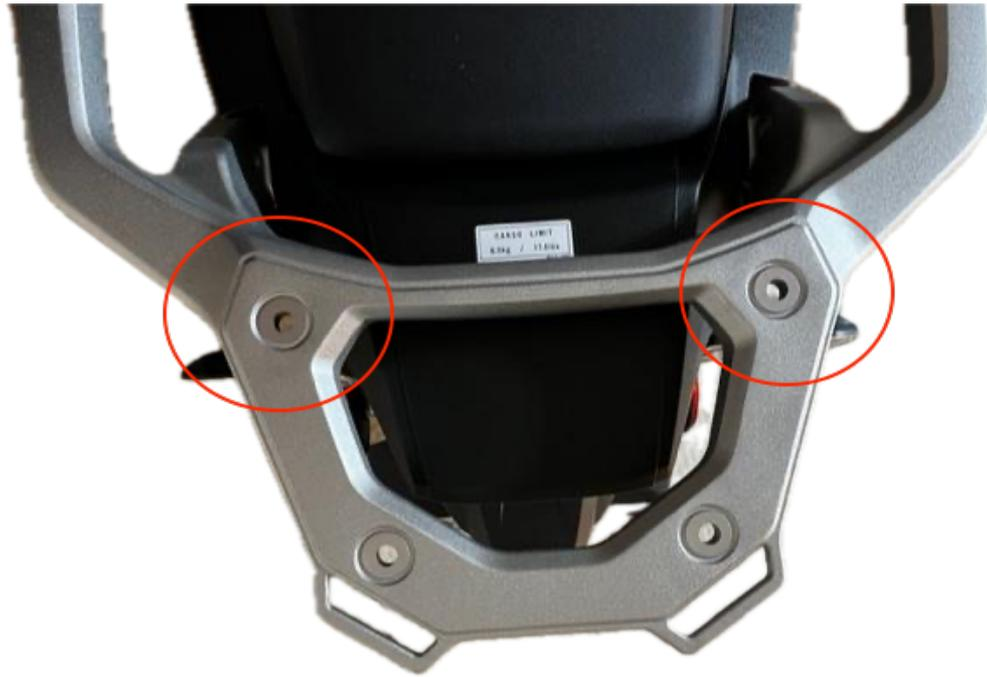
**Step 1** Install the 22 x 13 long aluminum spacers at the front of the OEM rack in the location shown.
