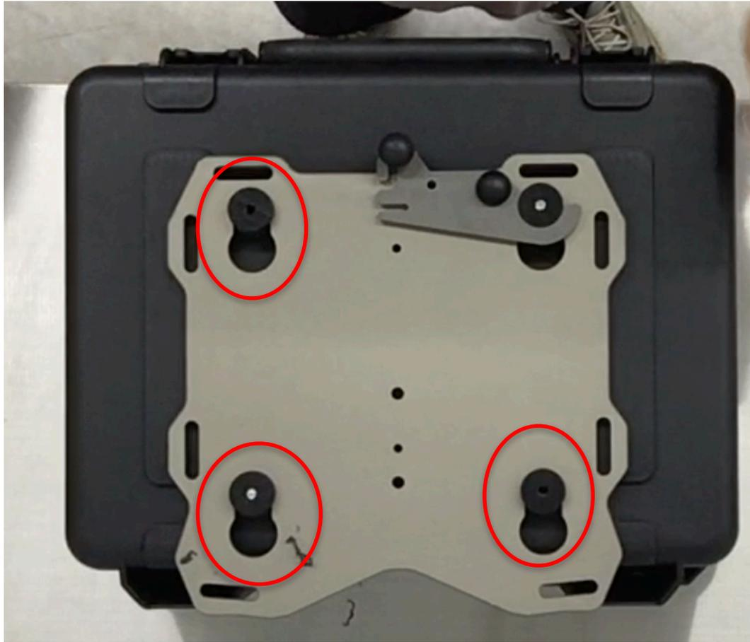
**Step 21** Attach the second puck to the case with the M8 hardware. Place the Slider rack on the case and latch it into position. With the ¼” drill bit use the 2 remaining pucks as drill guides and drill the last two ¼” holes.
