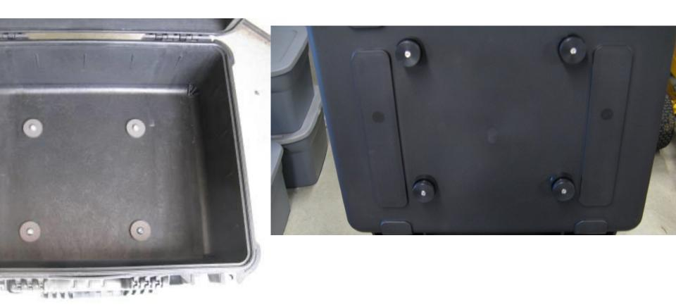
**Step 27** Install all pucks onto the case using the M8 flat washers and M8 button head cap screws. Lightly snug the puck screws at this time, later they will be fully tightened.
