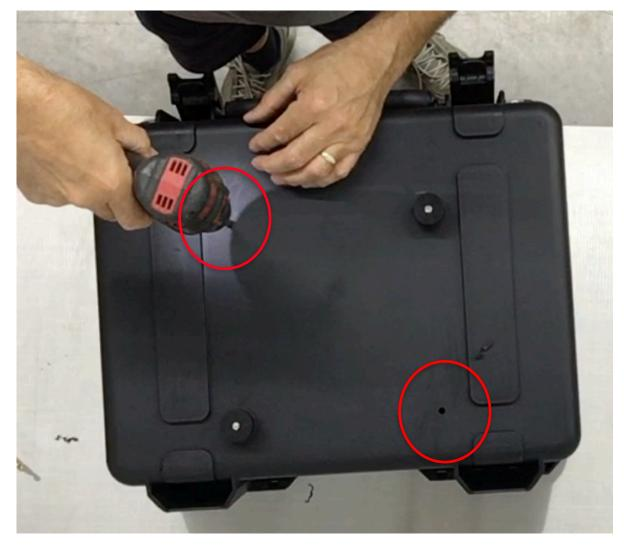
**Step 26** Remove the Slider rack and pucks from the case. Use the 21/64" drill bit and electric drill to enlarge the last 2 1/4" pilot holes.
