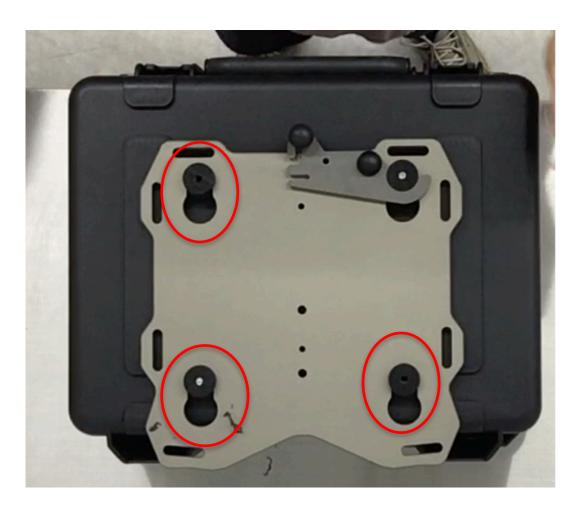
**Step 25** Attach the second puck to the case with the M8 hardware. Place the Slider rack on the case and latch it into position. With the  $\frac{1}{4}$ " drill bit use the 2 remaining pucks as drill guides and drill the last two  $\frac{1}{4}$ " holes.
