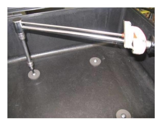
**Step 30** Torque the puck screws to 9 ft.lb. or 12.2 Nm.
