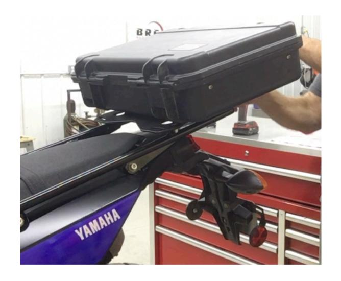
**Step 29** Install the case onto rack and latch it into place with the cam lever.
