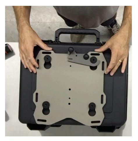
Step 17 Place the case on a table or other work surface. If the plate is still attached to the motorcycle loosen the RH & LH M8 socket head cap screws. Remove the 6 flat head screws and nuts holding the Slider plate onto the mounting tubes. Place the Slider plate with the pucks installed on the case.
