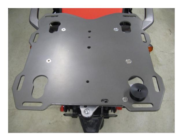
**Step 14** Install one of the black plastic pucks into the key hole with the cam lever. Lock the puck into place with the cam lever. This will be referred to as the "Master Puck" Note: Remove the large washer and screw from the puck before putting into the plate. The screws and washers are installed into the pucks for shipment as part of our QA process.
