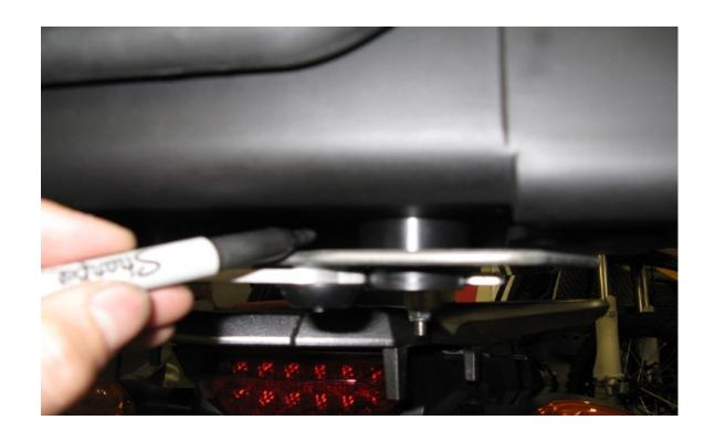
**Step 16** Position the case on top of the pucks. Determine the for/aft location (side to side will be determined later). Position the box as far forward as possible without interfering with passenger comfort. Also consider if you will be placing any gear on the seat or if you want to be able to remove the seat with the box in place. Use a marker to mark the master puck location on the box.
