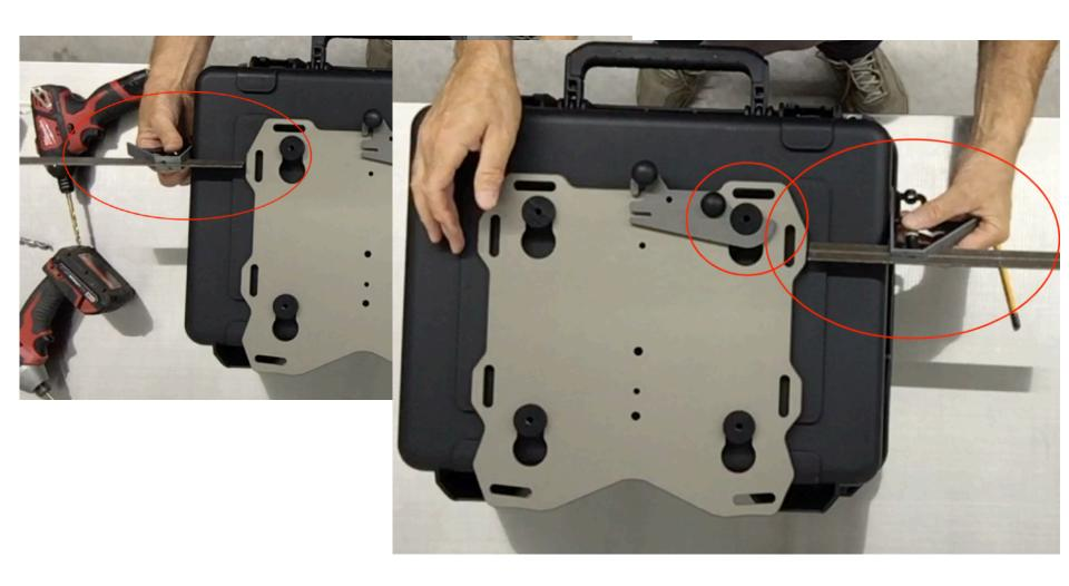
**Step 18** Locate the puck marker on the case and align the master puck with the mark as it was on the bike. Adjust the box side to side and make any final adjustments to the location.
