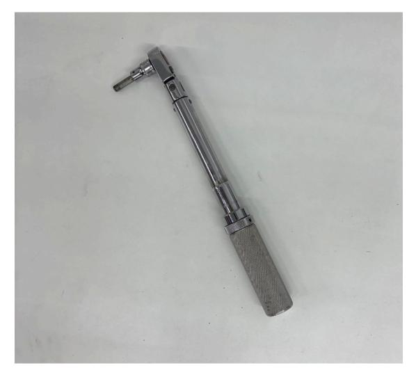
**Step 24** Use a M6 hex wrench and torque wrench to torque the four M8 screws to 26 Nm (19ftlb).
