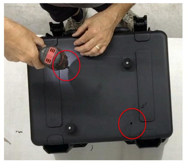
**Step 20** Remove the Slider rack and pucks from the case. Use the 21/64" drill bit and electric drill to enlarge the last 2 1/4" pilot holes.
