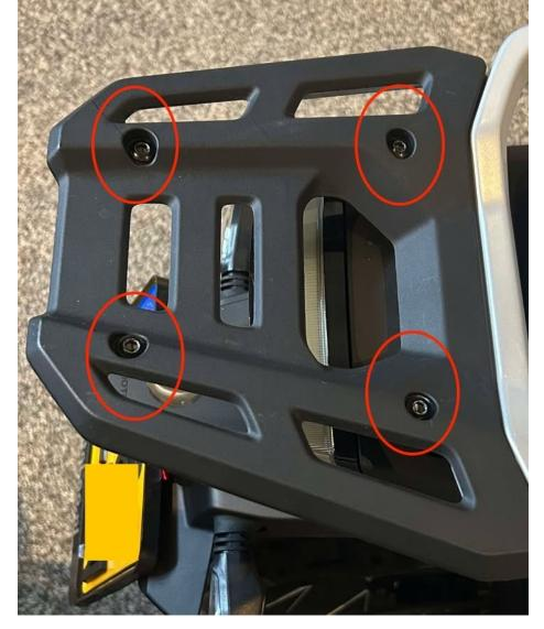
**Step 1** Using a 5mm hex bit (Allen wrench) remove the four M5 screws holding the plastic cover on. The plastic cover will not be used with the Slider rack.
