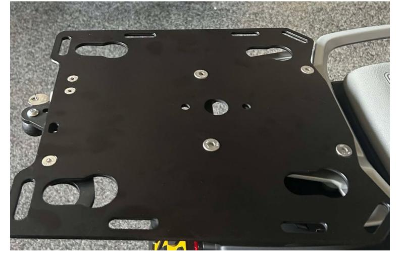
**Step 6** Place the Slider plate on top of the OEM rack and insert the two long M8 x 55 flat head screws through the plate and the spacers at the front two mounting holes. Insert the two short M8 x 35 screws at the rear mounting holes. Using your fingers thread the screws 3-4 turns before using a 6mm hex wrench to tighten. Final torque will be 26 Nm (19ftlb). **Note:** Apply blue 242 Loctite or equivalent to threads when installing the screws for the final time at **Step 24**.
