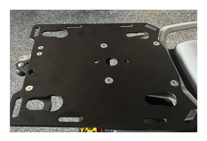
**Step 23** Follow steps 3 - 6 and re-install the plate onto the OEM rack.
