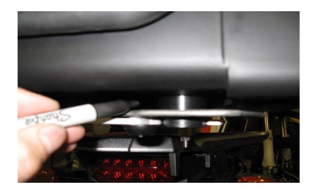
**Step 10** Position the case on top of the pucks. Determine the for/aft location (side to side will be determined later). Position the box as far forward as possible without interfering with passenger comfort. Also consider if you will be placing any gear on the seat or if you want to be able to remove the seat with the box in place. Use a marker to mark the master puck location on the box.
