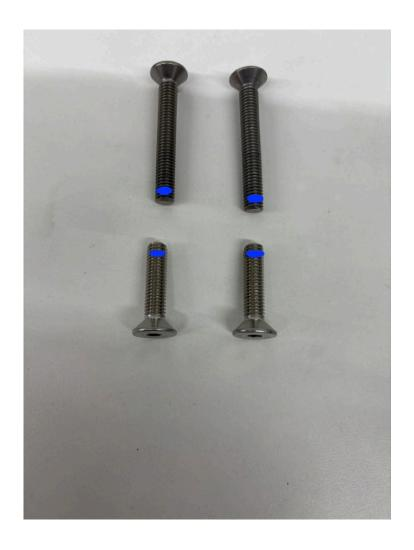
**Step 22** Apply blue 242 Loctite or equivalent to the four M8 screws that hold the Slider plate to the OEM rack.
