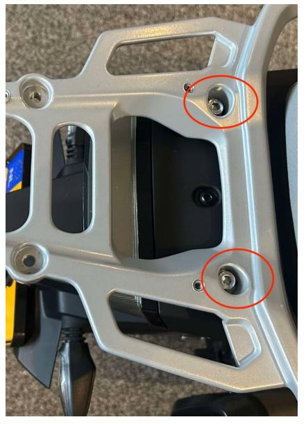
Step 2 Using a 6mm hex wrench (Allen wrench) remove the two M8 fasteners.
