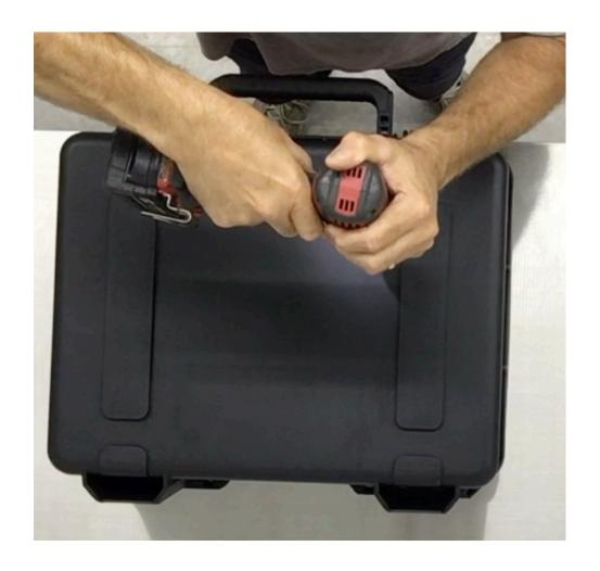
**Step 14** Remove the Slider plate from the case. Use the 21/64" drill bit and electric drill to enlarge the ½" pilot hole.
