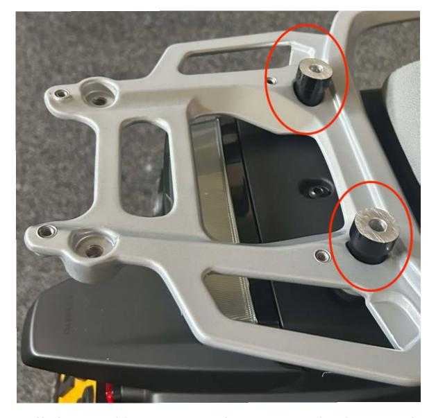
**Step 3** Install the two 22 mm stepped spacers in the front pockets as shown. **Note:** Small diameter fits into the pocket.
