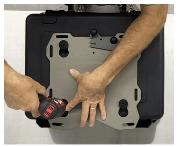
**Step 17** With the ¼" drill bit, use the puck diagonally across from the master puck as a drill guide and drill a second pilot hole in the case.
