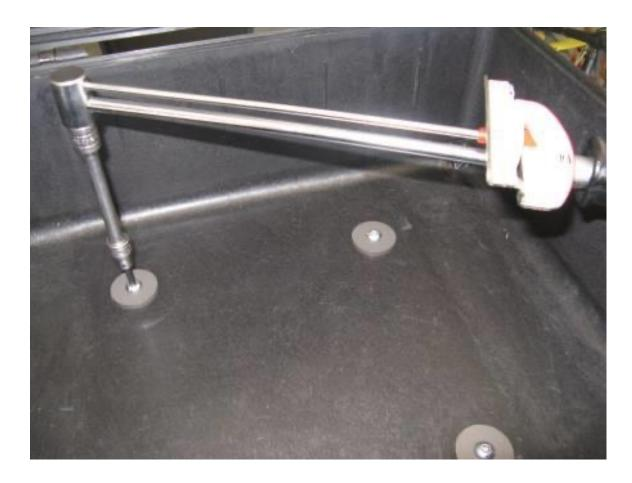
**Step 26** Torque the puck screws to 9 ft.lb. or 12.2 Nm.
