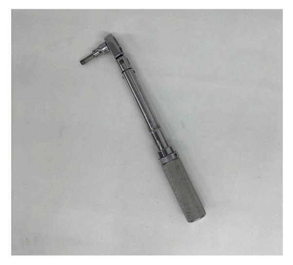
**Step 7** Use a M6 hex wrench and torque wrench to torque the four M8 screws to 26 Nm (19ftlb). **Note:** if you will be removing the plate for case drilling in **Step 13** do not torque the screws at this time. Final torque will be done in **Step 26**.
