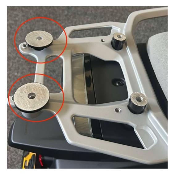
**Step 5** Stack the 41 x 5 mm aluminum spacers on top of the 16 x 15 mm aluminum spacers. **Note:** Make sure the uncoated side on the 41mm spacer is facing upward as shown.
