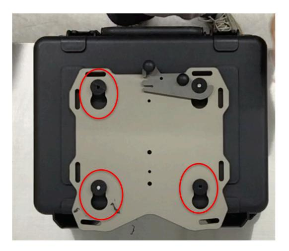
**Step 19** Attach the second puck to the case with the M8 hardware. Place the Slider rack on the case and latch it into position. With the  $\frac{1}{4}$ " drill bit use the 2 remaining pucks as drill guides and drill the last two  $\frac{1}{4}$ " holes.
