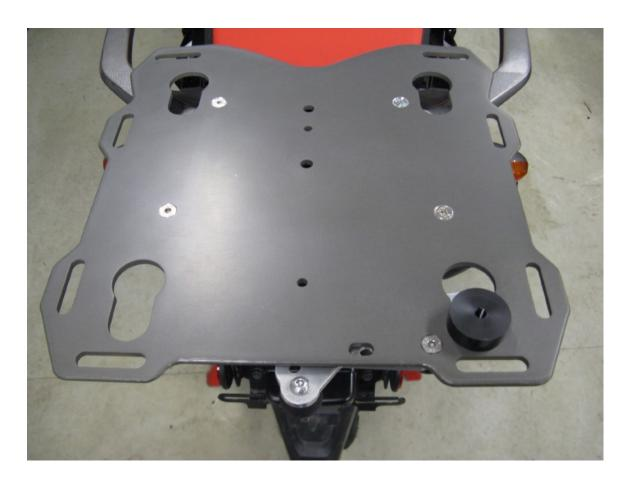
**Step 8** Install one of the black plastic pucks into the key hole with the cam lever. Lock the puck into place with the cam lever. This will be referred to as the "Master Puck" Note: Remove the large washer and screw from the puck before putting into the plate. The screws and washers are installed into the pucks for shipment as part of our QA process.
