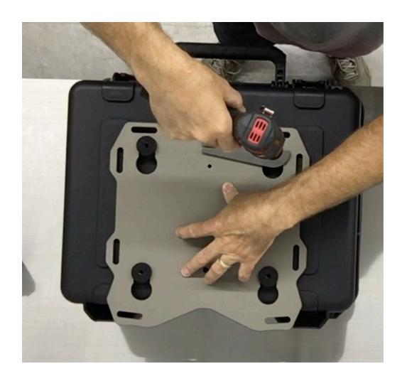
Step 13 With one hand apply downward force on the Slider plate, use your other hand to drill the case. With a ¼" drill bit and electric drill use the master puck as a drill guide and drill a pilot hole through the box.
