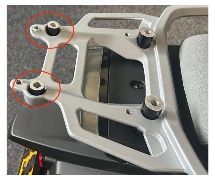
**Step 4** Insert the two 16 x 15 mm spacers into the rear pockets as shown.
