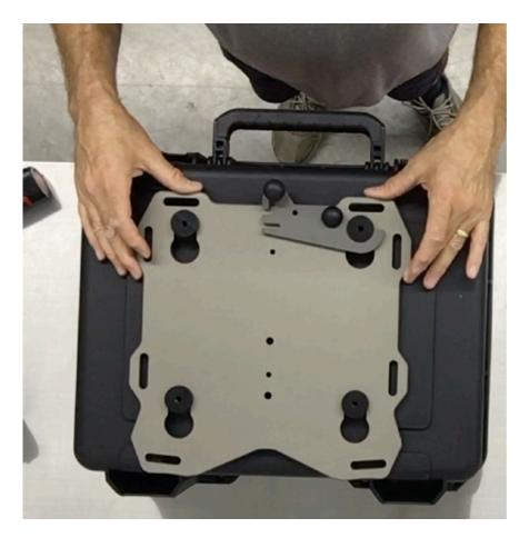
**Step 11** Place the case on a table or other work surface. Remove the 4 flat head screws and nuts holding the Slider plate onto the OEM rack. Place the Slider plate with the pucks installed on the case.
