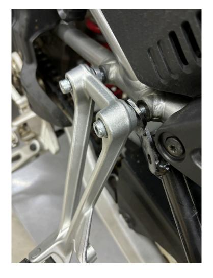
**Step 9a** Insert one screw through the pannier front mounting tab and thread into the rear subframe hole 3 to 4 revolutions. Thread the other screw into the forward subframe hole 3 to 4 revolutions as shown in the photo. Do not fully tighten the screws at this time.
