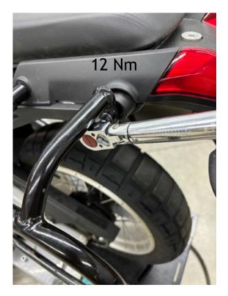
**Step 13** Torque LH mid mount and LH front mount M8 screws to 27 Nm (20 ftlb). Torque the LH rear mount M6 screw to 12 Nm (9 ftlb). Repeat for RH pannier. **Note:** For proper performance all mounting fastener's final tightening must be done with an accurate torque wrench.
