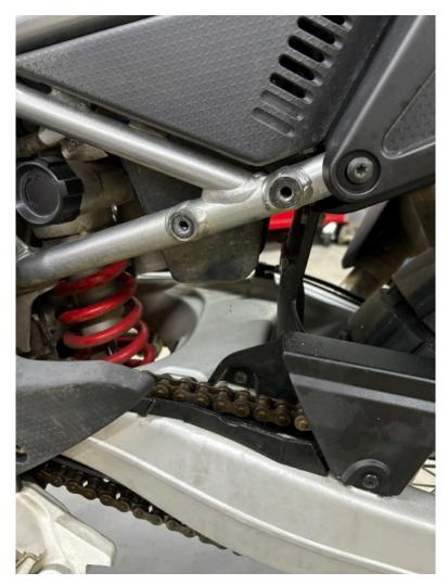
**Step 3** Using a 10mm socket wrench remove the two M8 screws holding the LH foot peg bracket to the subframe. Repeat for the RH foot peg bracket.
