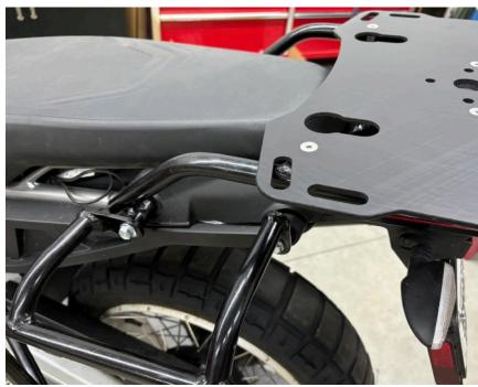
**Step 4** Insert the 25 mm stepped aluminum spacer with small diameter facing inward.
