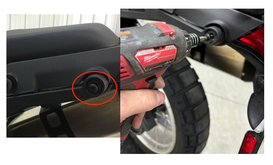
**Step 2** Locate the M6 LH pannier mount fastener, use a T30 bit to remove. Repeat on the RH side.
