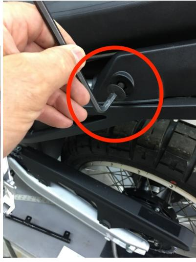
**Step 1** Locate the left hand (LH) M8 pannier mount fastener, use a 6mm hex wrench to remove. Repeat for the RH side.
