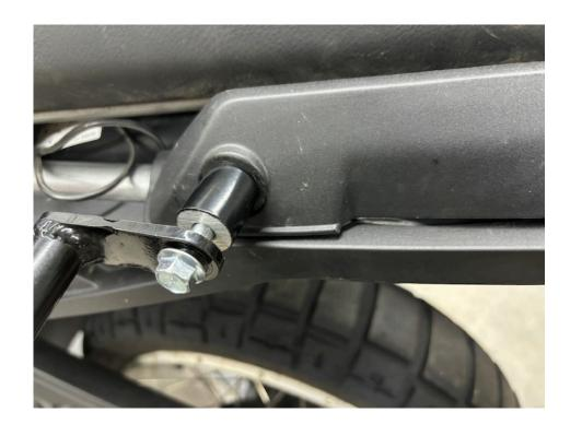
**Step 5** Insert the M8 x 50 flange head screw through the LH pannier middle mount and through the stepped spacer and hand thread 3 - 4 revolutions. **Note:** Do not tighten at this time!
