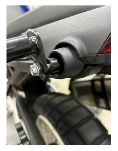
**Step 7** Insert the 6mm x 6mm aluminum spacer into the LH rear most subframe opening.
