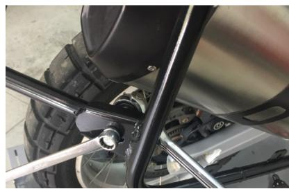
**Step 12** Center the rear cross bar and use 12mm and 13mm wrenches to snug the two cross bar screws and nuts.
