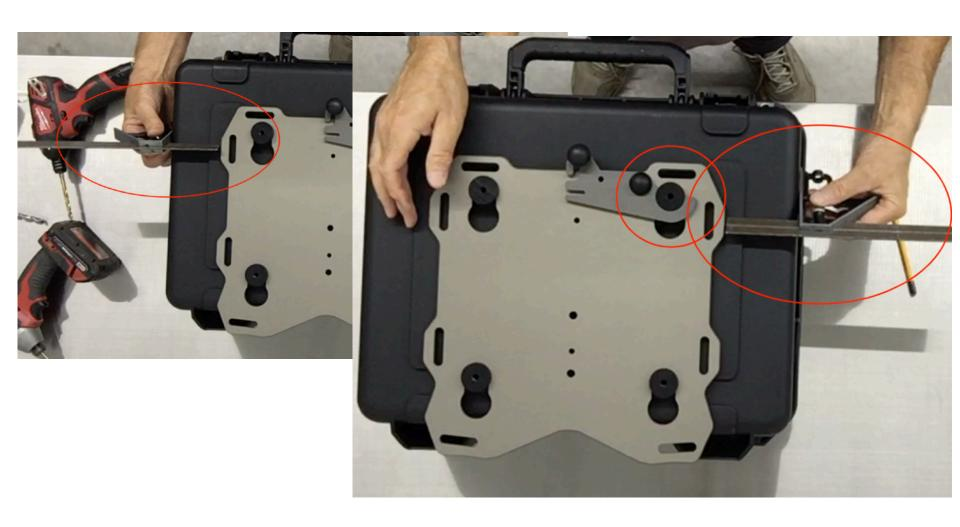
**Step 14** Locate the puck marker on the case and align the master puck with the mark as it was on the bike. Adjust the box side to side and make any final adjustments to the location.
