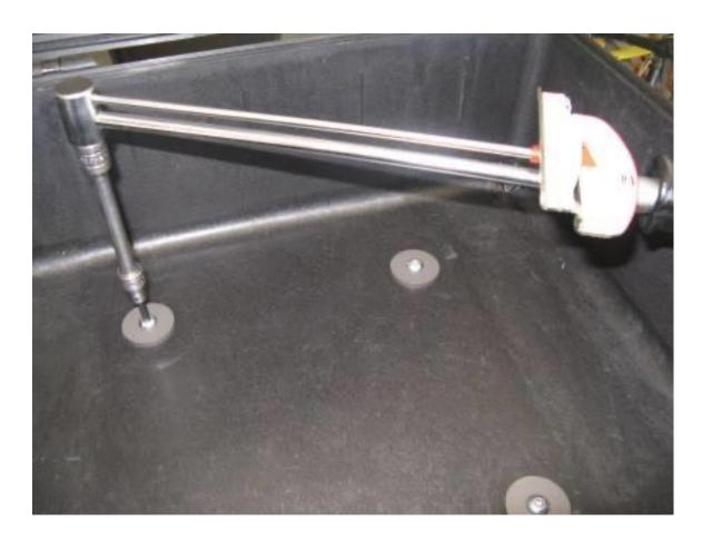
**Step 27** Torque the puck screws to 9 ft.lb. or 12.2 Nm.
