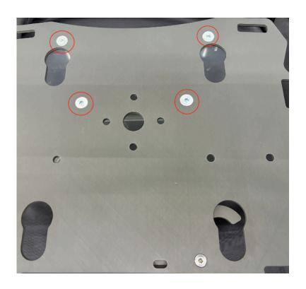
**Step 3** Place the Slider plate on top of the OEM rack and insert the the four M8 flat head screws through the plate and the spacers.
