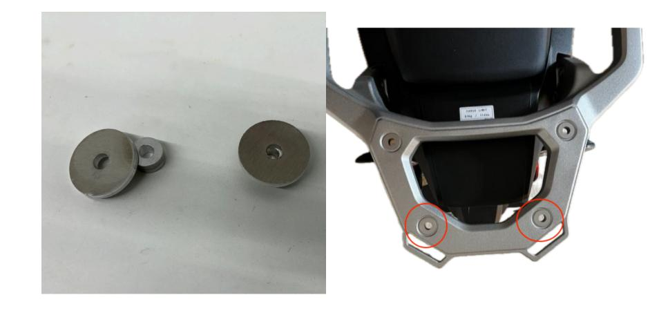
**Step 2** Stack the 41 x 5 mm aluminum spacers on top of 22 x 8 mm aluminum spacers. Place a spacer stack over each of the rear holes as shown.
