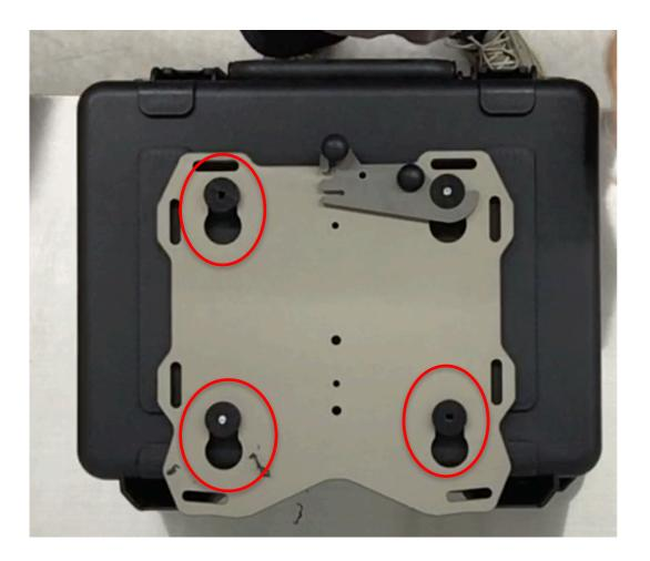
**Step 21** Attach the second puck to the case with the M8 hardware. Place the Slider rack on the case and latch it into position. With the ¼" drill bit use the 2 remaining pucks as drill guides and drill the last two 1/4" holes.
