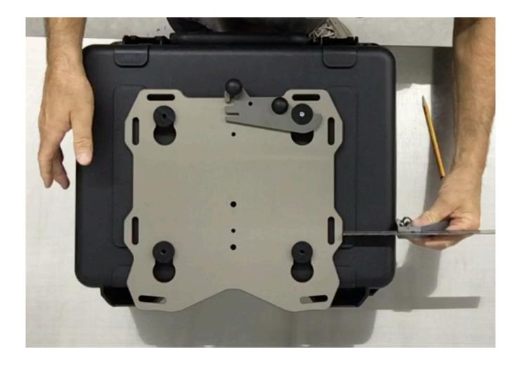
**Step 22** Place the Slider plate with the other 3 pucks onto the master puck and latch it into position. Square up the plate and box to each other (last chance).
