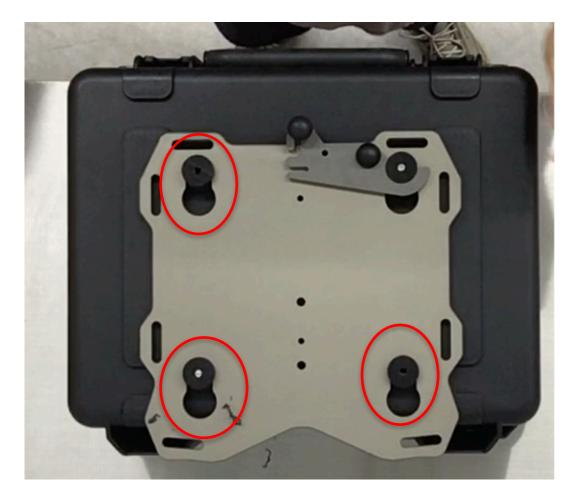
**Step 25** Attach the second puck to the case with the M8 hardware. Place the Slider rack on the case and latch it into position. With the <sup>1</sup>/<sub>4</sub>" drill bit use the 2 remaining pucks as drill guides and drill the last two 1/4" holes.
