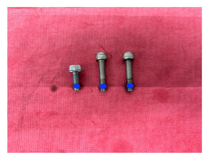
**Step 4** Apply Blue 242 Loctite or equivalent to the threads of the M8 x 25 flange head cap screw and the two M8 X 35 socket head cap screws (SHCS).
