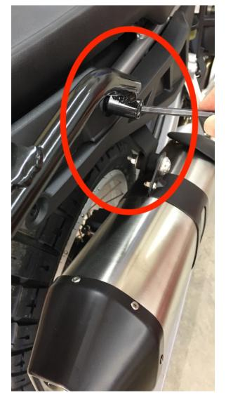
**Step 8** Attach the front of the RH mounting tube with a M8 x 35 SHCS. Do not tighten at this time, turn the screw 3 to 4 revolutions. **Note:** make certain the small diameter on the boss passes through the the hole in the OEM plastic
