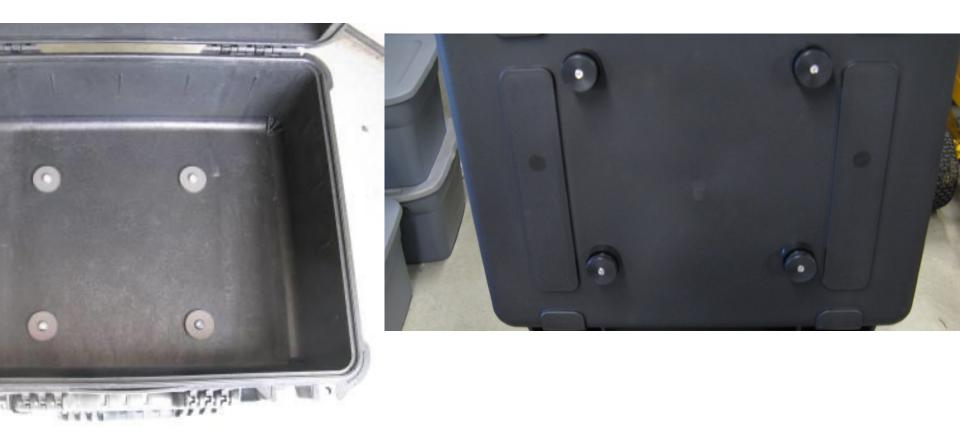
**Step 27** Install all pucks onto the case using the M8 flat washers and M8 button head cap screws. Lightly snug the puck screws at this time, later they will be fully tightened.
