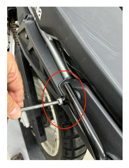
**Step 10** Attach the front of the LH mounting tube with a M8 x 35 SHCS. Do not tighten at this time, turn the screw 3 to 4 revolutions. **Note:** make certain the small diameter on the boss passes through the the hole in the OEM plastic
