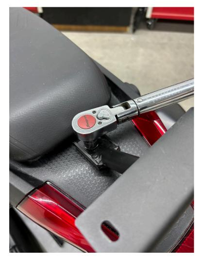
Step 5 Using the M8 x 20 flange head cap screw attach the rear bracket. Square the bracket to the bike. Tighten and torque the cap screw to 20 ft. lb.
