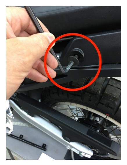
**Step 2** Remove the RH & LH OEM M8 screws. These screws will **not** be used with the BRE Slider rack.
