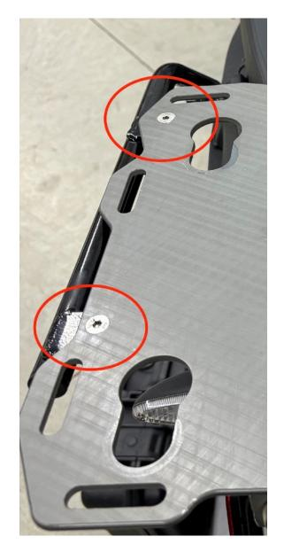
**Step 9** Attach the rear of the LH mounting tube to the Slider plate with two M6 x 18 flat head screws and M6 lock nuts. Hand tighten the screws at this time.
