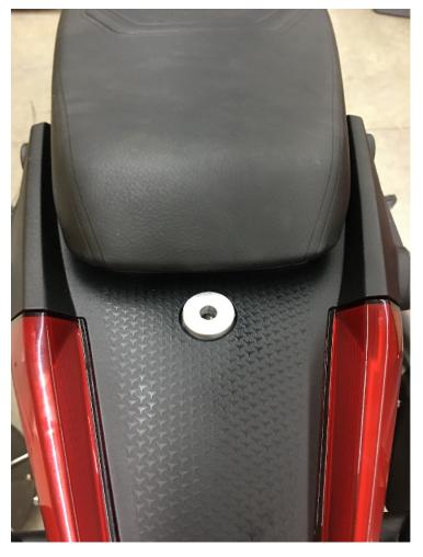
Step 3 Insert stepped aluminum spacer with small diameter facing downward.
