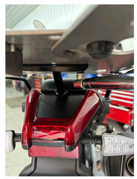
**Step 11** Torque the 2 center M6 x 18 flat head screws to 9 ft. lbs.
