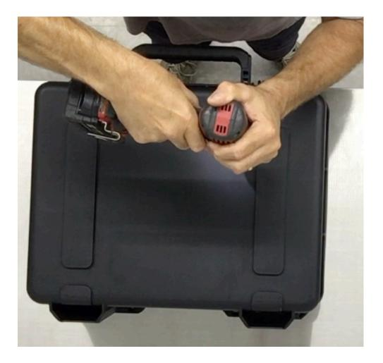
Step 20 Remove the Slider plate from the case. Use the 21/64" drill bit and electric drill to enlarge the  $\frac{1}{4}$ " pilot hole.
