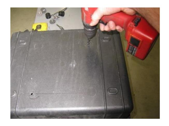
**Step 24** Remove the plate and pucks from the box. Use the 21/64" drill bit and electric drill to enlarge the pilot hole.
