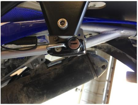
**Step 11** Snug the M8 and M10 tube mounting bolts so their is no clearance between the mounting brackets and the subframe but do not apply final torque.
