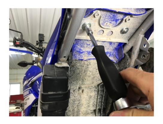
**Step 1** Unthread the 2 bolts that retain the seat and remove the seat.
