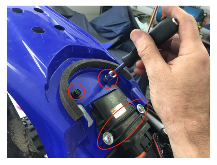
**Step 2** Remove the 2 bolts that retain the fender and remove the rubber o-ring that retains the ECU.
