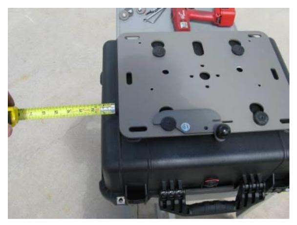
**Step 18** Locate the puck marker on the box and align the master puck up with the mark as it was on the bike.
