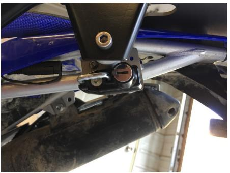
**Step 13** Perform final tighten/torque on M8 and M10 bolts.
