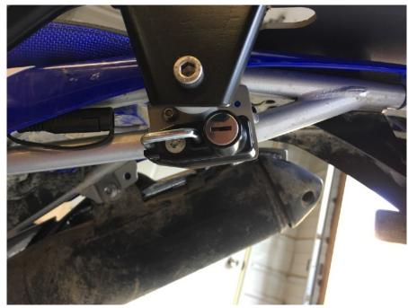
**Step 7** Attach the left hand BRE tube with the M8 x 70 screw. The screw will pass through the tube bracket, the large diameter spacer, the small diameter spacer and the helmet lock relocation bracket. Hand tighten the screw at this time. **Note:** Installing the OEM helmet lock is optional.
