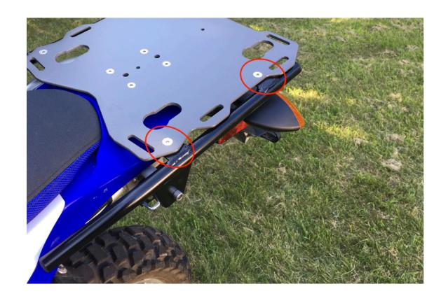
**Step 8** Insert two M6 x 18 flat head screws into the plate and through the mounting tabs on the left hand BRE tube. Install M6 washers and locking nuts do not tighten nuts at this time.
