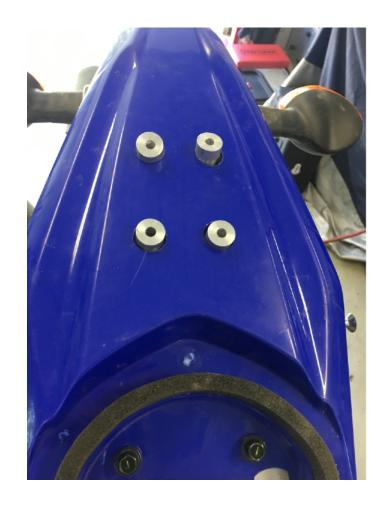
**Step 4** Reinstall the rear fender on the motorcycle and insert the four long 19mm aluminum spacers into the fender holes. Tighten the fender mounting screws and reinstall the ECU o-ring.
