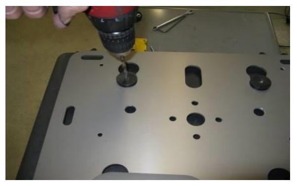
**Step 25** Bolt the second puck to the box. Place the plate on the box and latch it into position. With the ¼" drill bit use the 2 remaining pucks as drill guides and drill the last 2 pilot holes.
