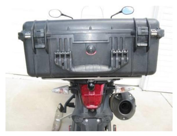
Step 29 Install the box onto rack and latch it into place with the cam lever.
