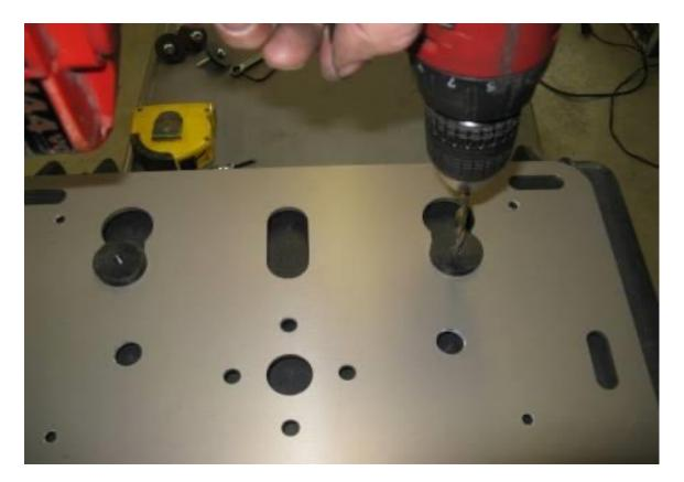
**Step 23** With the ¼" drill bit, use the puck diagonally across from the master puck as a drill guide and drill a second pilot hole in the box.
