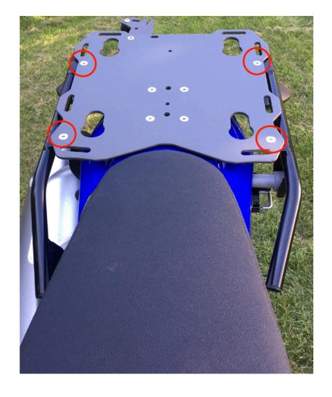
**Step 12** Tighten all 4 M6 flat head screws with 4mm hex wrench and 10mm socket wrench.
