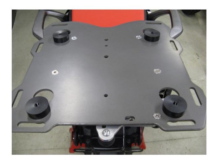
**Step 15** Insert the 3 remaining pucks into the keyholes in the plate.
