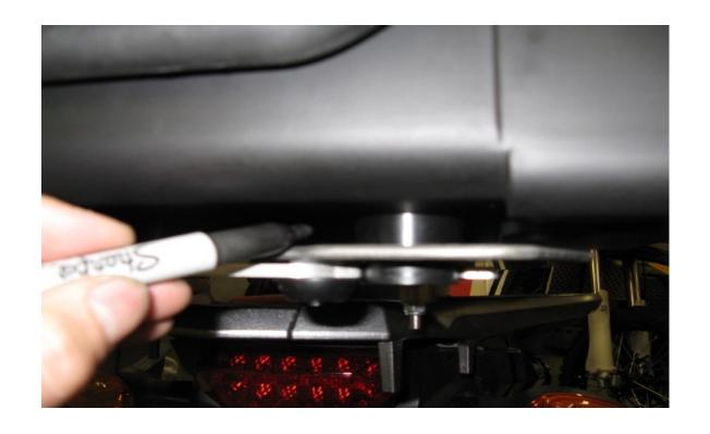
**Step 4** Position the case on top of the pucks. Determine the for/aft location (side to side will be determined later). Position the case as far forward as possible without interfering with passenger comfort. Also consider if you will be placing any gear on the seat or if you want to be able to remove the seat with the case in place. Use a marker to mark the master puck location on the case.
