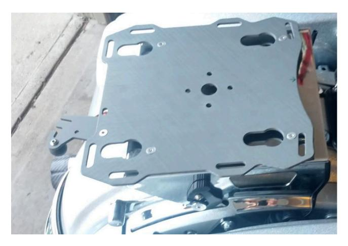
**Step 1** Install the BRE plate as shown with four M6 x 25 screws. The aluminum spacers go between the BRE plate and the Tour-Pak, the flat washers and lock nuts are located underneath the Tour-Pak.
