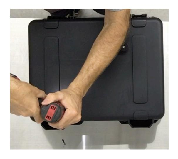
**Step 12** Remove the slider plate from the case and use the 121/64" drill bit to enlarge the second 1/4" pilot hole.
