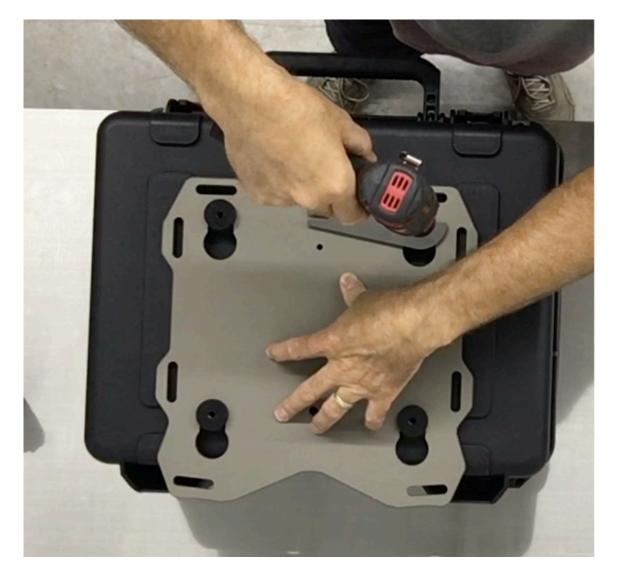
**Step 7** With one hand apply downward force on the Slider plate, use your other hand to drill the case. With a  $\frac{1}{4}$ " drill bit and electric drill use the master puck as a drill guide and drill a pilot hole through the box.
