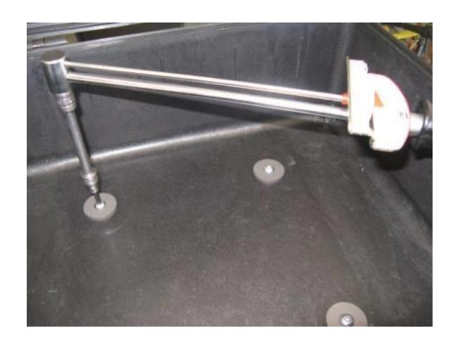
Step 19 Torque the puck screws to 9 ft. lbs. (12.2 Nm).
