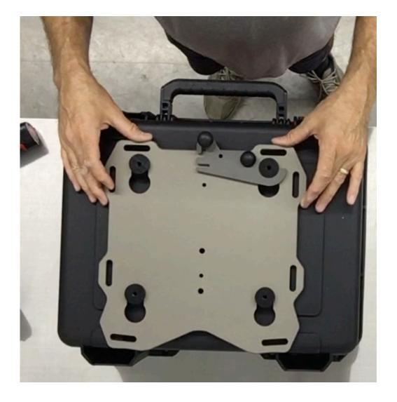
**Step 5** Place the case on a table or other work surface. Remove the 4 screws holding the Slider plate onto the motorcycle. Place the Slider plate with the pucks installed onto the case.
