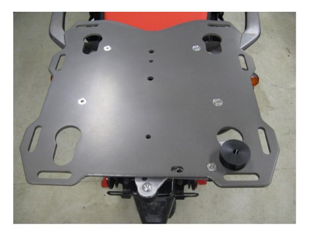
**Step 2** Install one of the black plastic pucks into the key hole with the cam lever. Lock the puck into place with the cam lever. This will be referred to as the "Master Puck"
