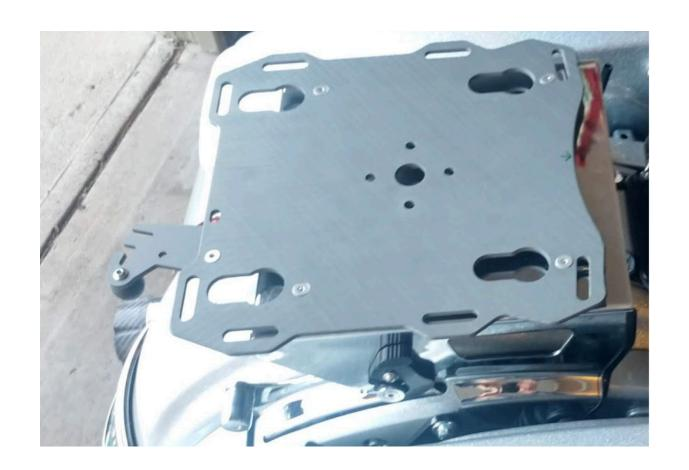
**Step 16** Re-install the Slider plate onto the Tour-Pak with the M6 x 25 flat head screws, aluminum spacers, flat washers and M6 lock nuts.
