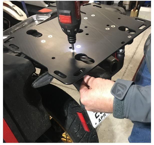
**Step 6** Use a 4mm driver and 10mm open end wrench to tighten all eight M6 lock nuts. **Note:** Clamp halves will be closed together when tightened correctly, do not over tighten.
