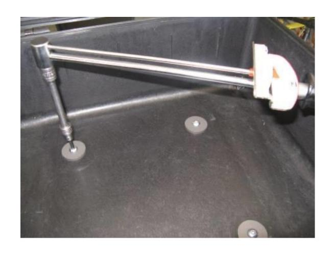
Step 24 Torque the puck screws to 9 ft. lbs. or 12.2 Nm.
