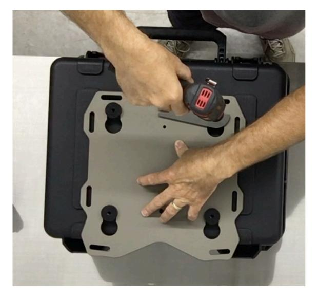
**Step 12** With one hand apply downward force on the Slider plate, use your other hand to drill the case. With a  $\frac{1}{4}$ " drill bit and electric drill use the master puck as a drill guide and drill a pilot hole through the box.
