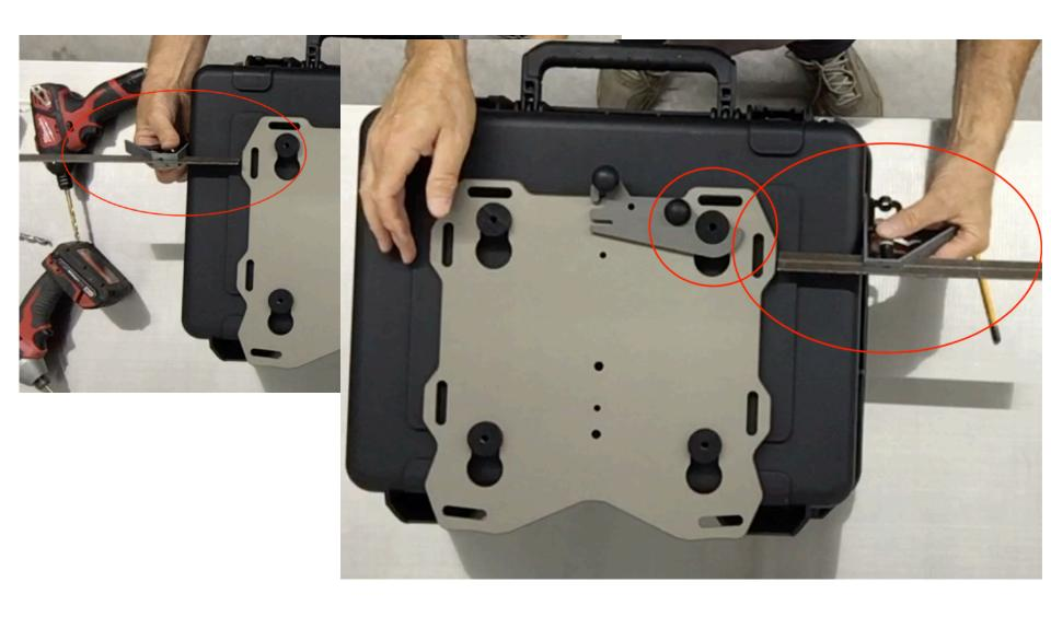
**Step 11** Locate the puck mark on the case and align the master puck with the mark as it was on the bike. Adjust the box side to side and make any final adjustments to the location.
