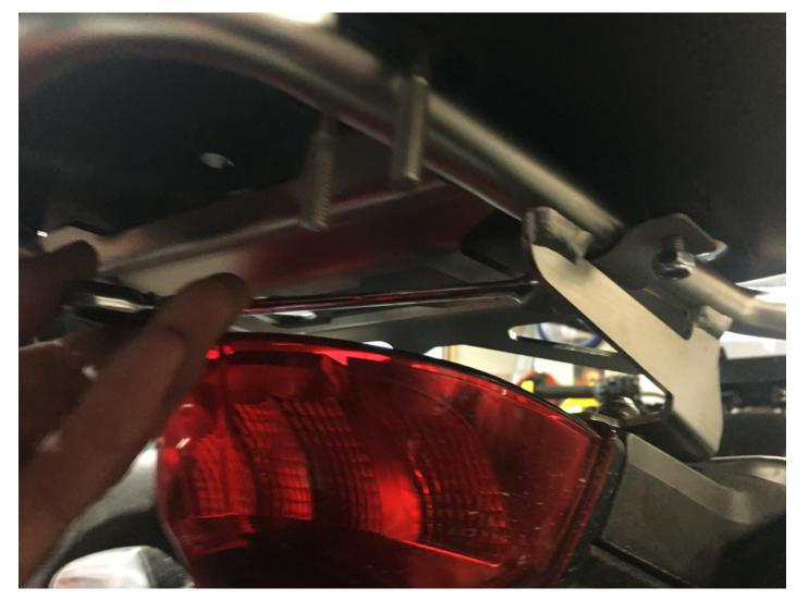
**Step 4** Thread the M6 lock nuts onto the front four flat head screws. **Tip:** Use an open end wrench with a piece of duct tape to help put the lock nut into position.
