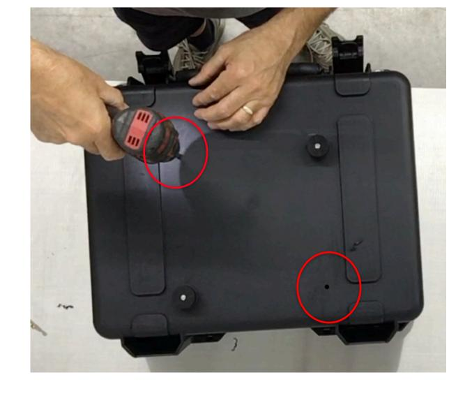
**Step 19** Remove the Slider rack and pucks from the case. Use the 21/64" drill bit and electric drill to enlarge the last 2 1/4" pilot holes.
