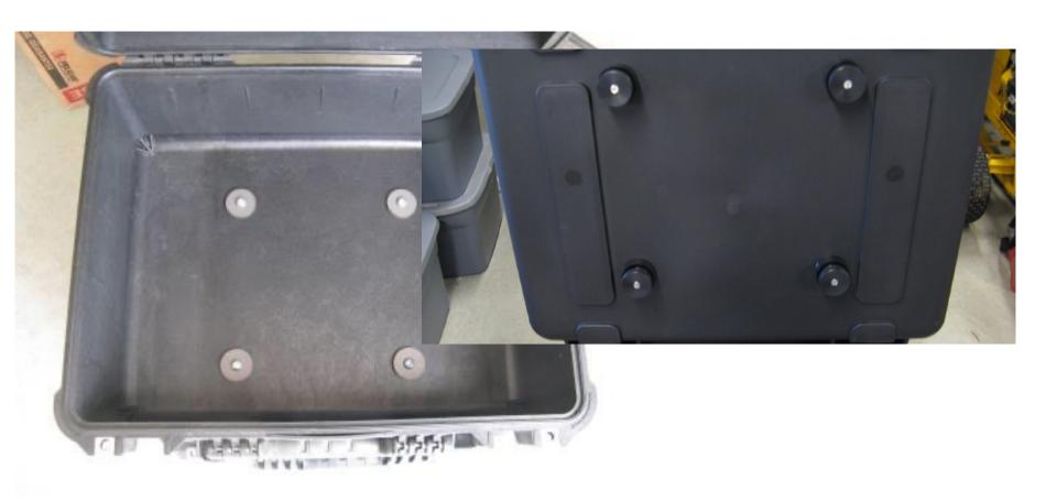
**Step 20** Install all pucks onto the case using the M8 flat washers and M8 button head cap screws. Lightly snug the puck screws at this time, later they will be fully tightened.
