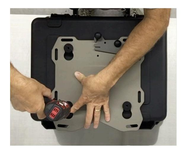
**Step 16** With the  $\frac{1}{4}$ " drill bit, use the puck diagonally across from the master puck as a drill guide and drill a second pilot hole in the case.
